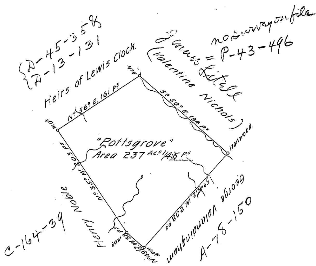
A Draught of a Survey called "Potts grove" situate on the Waters of Robinsons Run in Washington County, containg 237 Ac<sup>s</sup> 45 P<sup>s</sup> and the Allow<sup>c</sup>e for Highways 85<sup>s</sup>, executed Sept<sup>r</sup> ye 2<sup>d</sup> 1786, in Pursuance of a Warrant granted to Henry Potter for 250 Ac<sup>s</sup> dated June ye 5<sup>th</sup> 1786.
